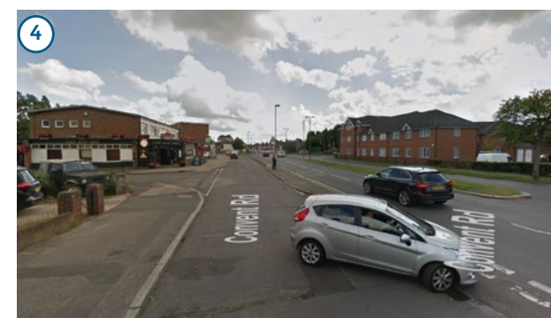
Figure 121. Covent Road east service road: poor footway surface quality, wide carriageway, narrow waiting area at the bus stop, and vehicles exiting on the main road at several locations increasing the risk of collision.
