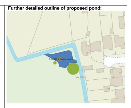
The proposed pond will act as both a flood alleviation mechanism and drought resilience mechanism. Additionally, it will be designed with the target of increasing biodiversity and aiding nature recovery within the area whilst also acting as a carbon sink.
