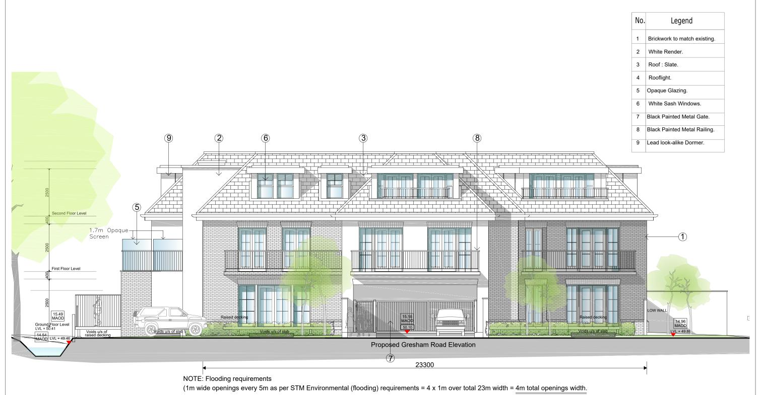
Total achieved within metal entrance gates to undercroft car parking area = 6m gate width - indicative voids shown under ground floor slab = 2m x 200mm (x2) = 4m total = TOTAL 10M
