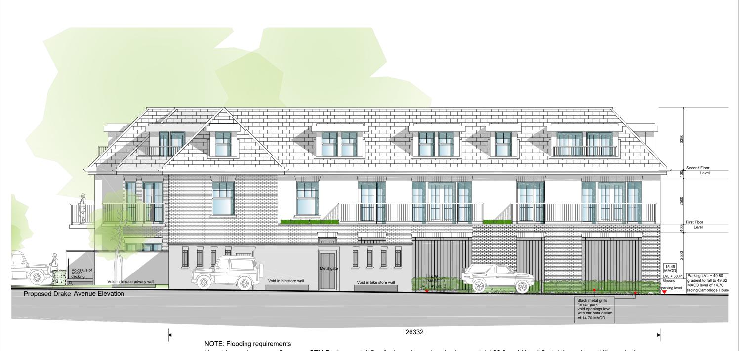
(1m wide openings every 5m as per STM Environmental (flooding) requirements = 4 x 1m over total 26.3m width = 4.5m total openings width required.
